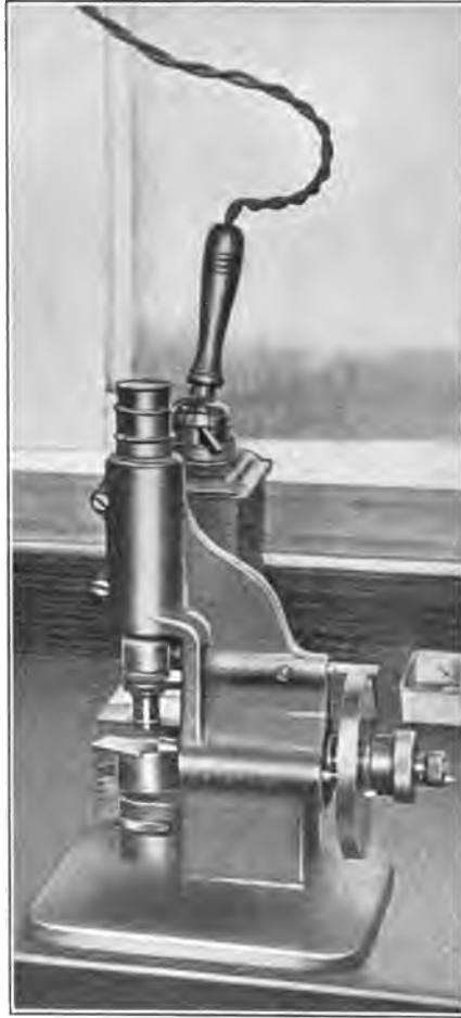
FIG. 165. — MICROSCOPE FOR INSPECTING DISPLAY MATRIX
